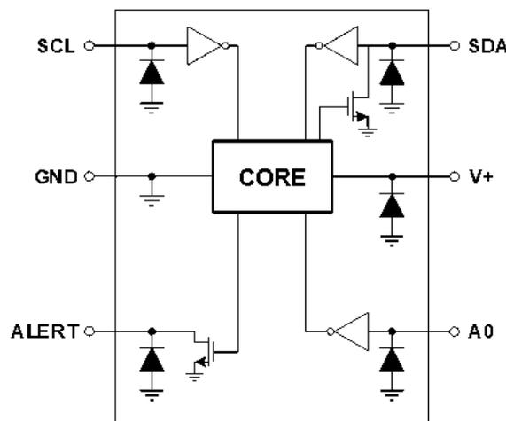
Figure 1. GD30TS112N Internal ESD Equivalent Circuit
