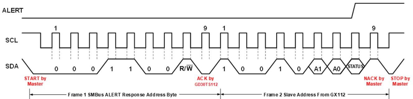
Figure 6. SMBus Alert Timing Diagram
