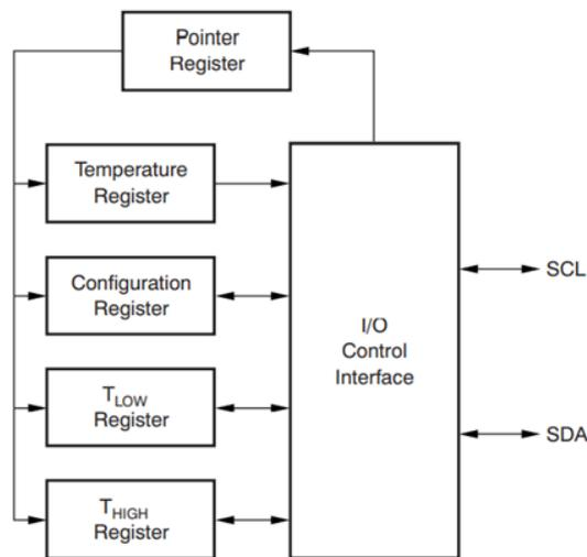
Figure 7. Internal Register Structure
