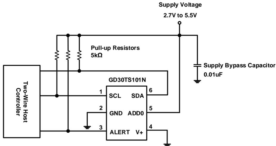
**Figure 8. Typical Connections of the GD30TS101N**
