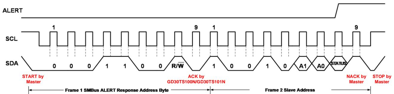
Figure 6. SMBus Alert Timing Diagram
