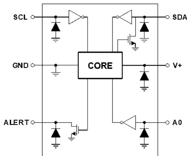
Figure 1. GD30TS101N Internal ESD Equivalent Circuit
