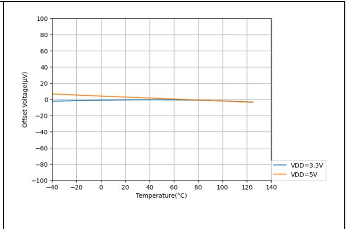
Figure 9. Offset Voltage vs. Temperature (FSR =  $\pm$  0.256V)
