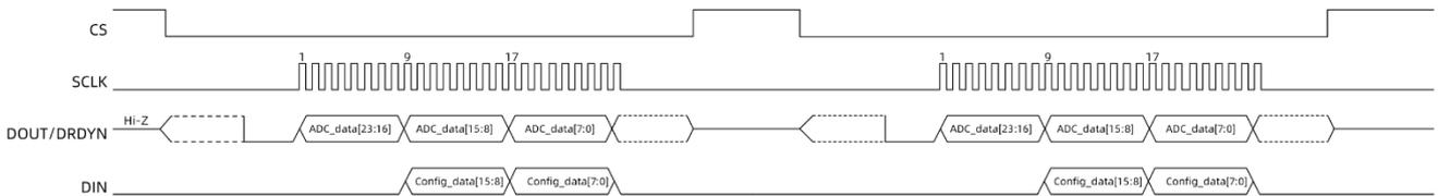
Figure 23. 24-Bit Data Transfer Cycle
