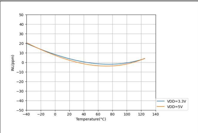
Figure 15. INL vs. Temperature (FSR =  $\pm 0.512V$ )
