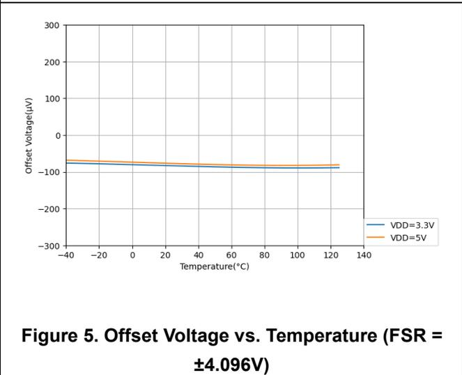
Figure 5. Offset Voltage vs. Temperature (FSR =  $\pm 4.096V$ )
