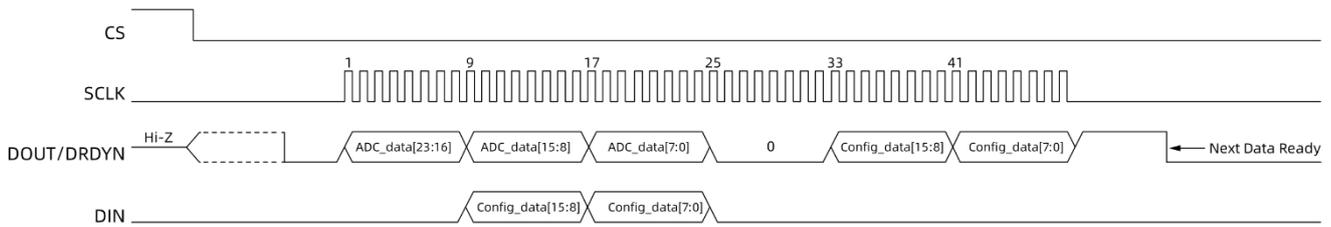
Figure 22. 24-Bit Data Transfer Cycle DIN Remains Low
