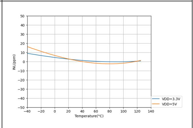
Figure 11. INL vs. Temperature (FSR =  $\pm$ 6.144V)
