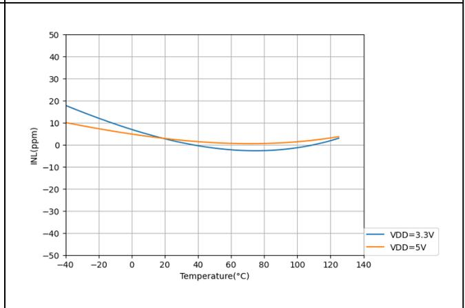
Figure 13. INL vs. Temperature (FSR =  $\pm$ 2.048V)
