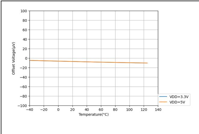
Figure 8. Offset Voltage vs. Temperature (FSR =  $\pm$  0.512V)
