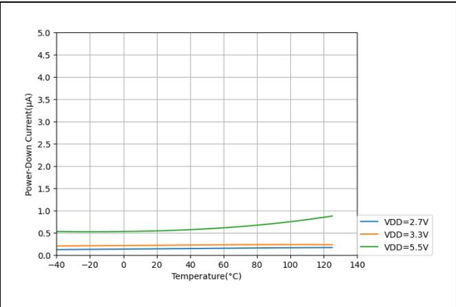
Figure 3. Power-Down Current vs. Temperature
