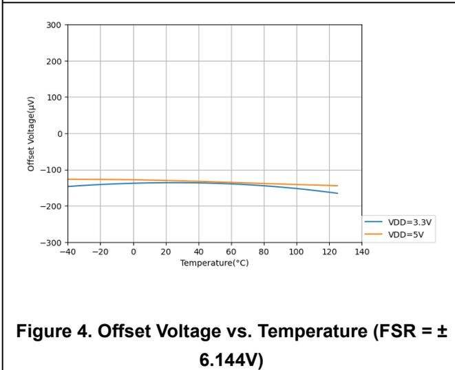
Figure 4. Offset Voltage vs. Temperature (FSR =  $\pm 6.144V$ )
