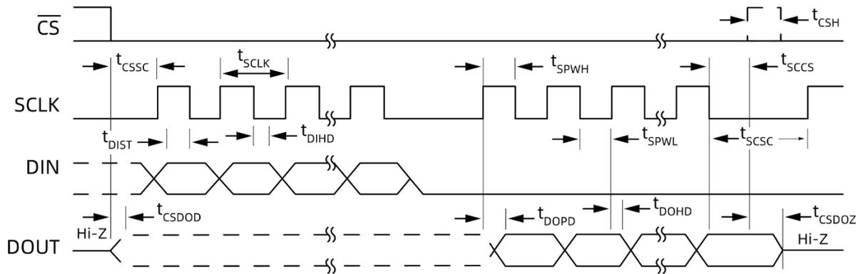
Figure 1. SPI Interface Timing
