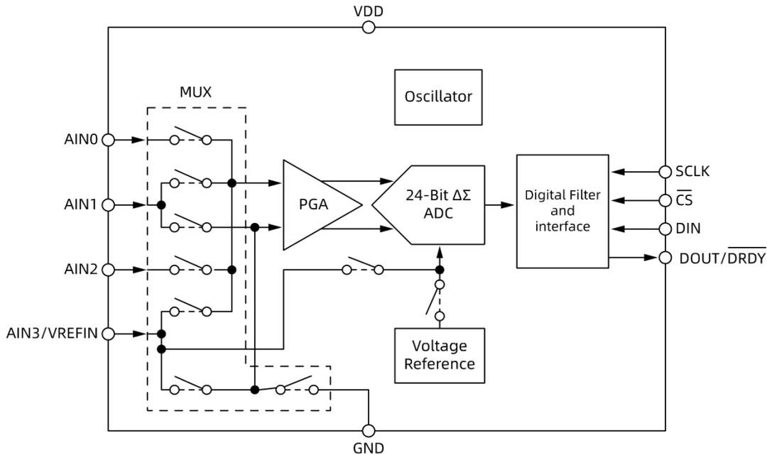
Figure 18. GD30AD3641 Block Diagram
