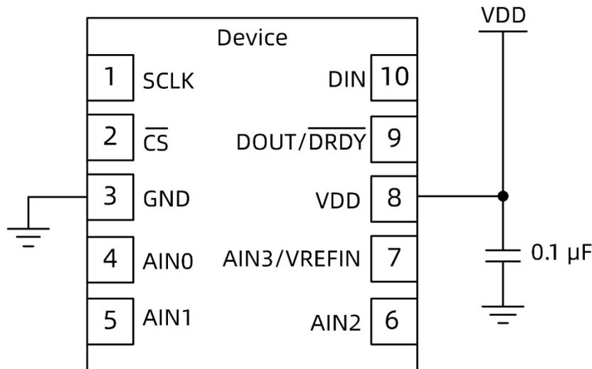
Figure 27. GD30AD3641 Power Supply Decoupling
