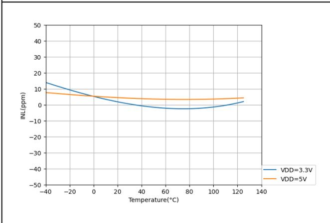
Figure 12. INL vs. Temperature (FSR =  $\pm$ 4.096V)
