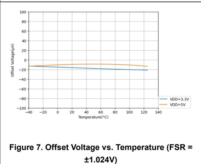
Figure 7. Offset Voltage vs. Temperature (FSR =  $\pm 1.024V$ )
