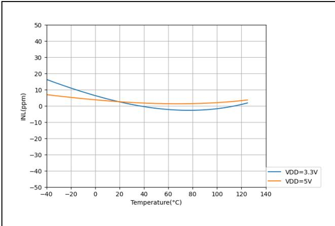
Figure 14. INL vs. Temperature (FSR =  $\pm 1.024V$ )
