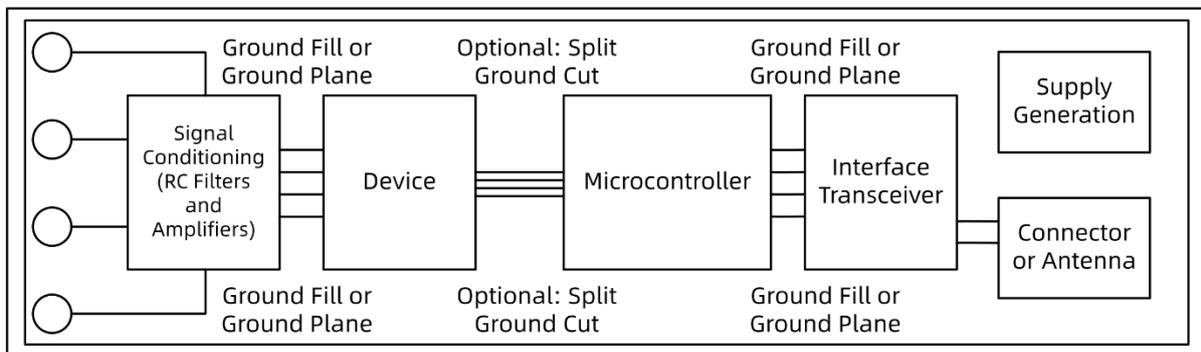
**Figure 28. System Component Placement**
