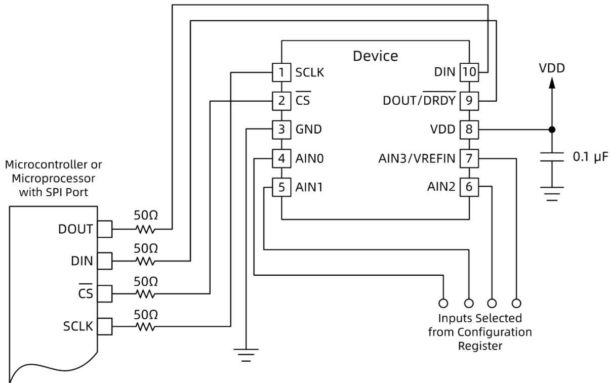
**Figure 24. Typical Connections for GD30AD3641**
