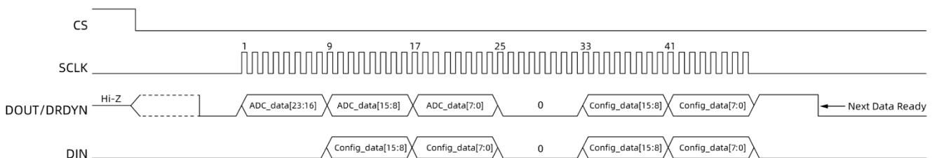
**Figure 21. 24-Bit Data Transfer Cycle-Configuration Register**
