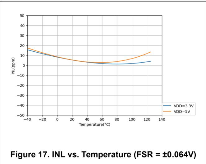
Figure 17. INL vs. Temperature (FSR =  $\pm 0.064V$ )
