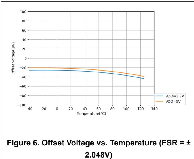
Figure 6. Offset Voltage vs. Temperature (FSR =  $\pm 2.048V$ )
