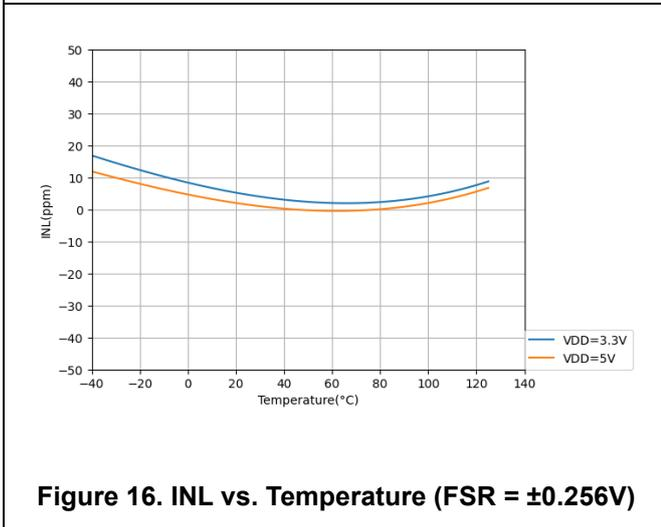
Figure 16. INL vs. Temperature (FSR =  $\pm 0.256V$ )
