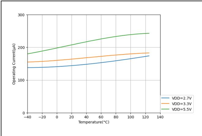
Figure 2. Operating Current vs. Temperature
