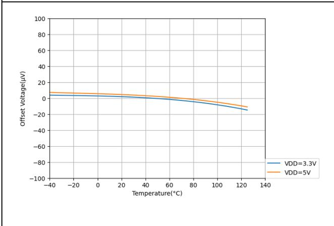
Figure 10. Offset Voltage vs. Temperature (FSR =  $\pm$  0.064V)
