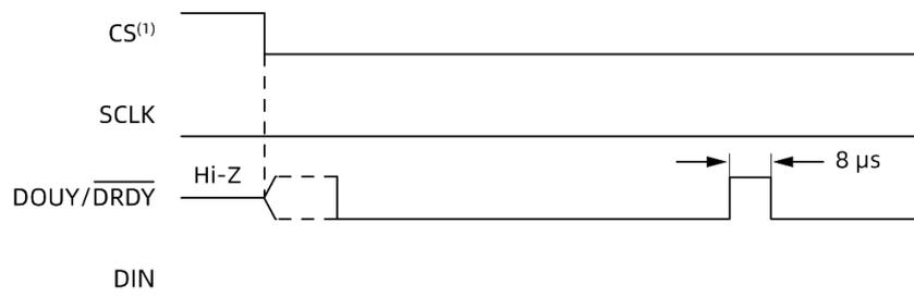
**Figure 20. Schematic Diagram of Continuous Conversion Mode without Data Reading DOUT/ $\overline{DRDY}$**
