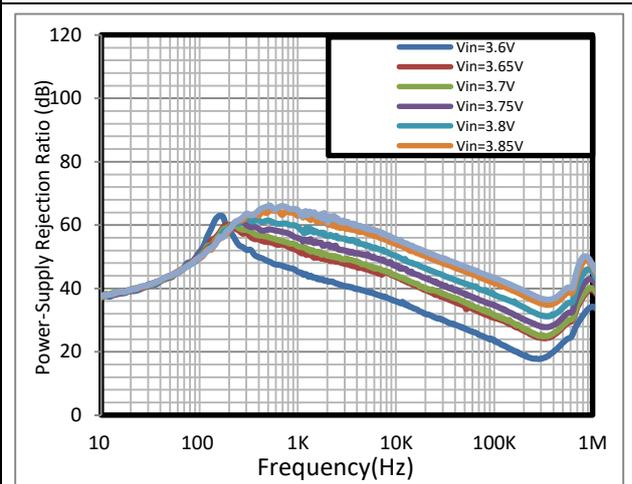
$V_{OUT} = 3.3\text{V}$ ,  $I_{OUT} = 1.2\text{A}$
