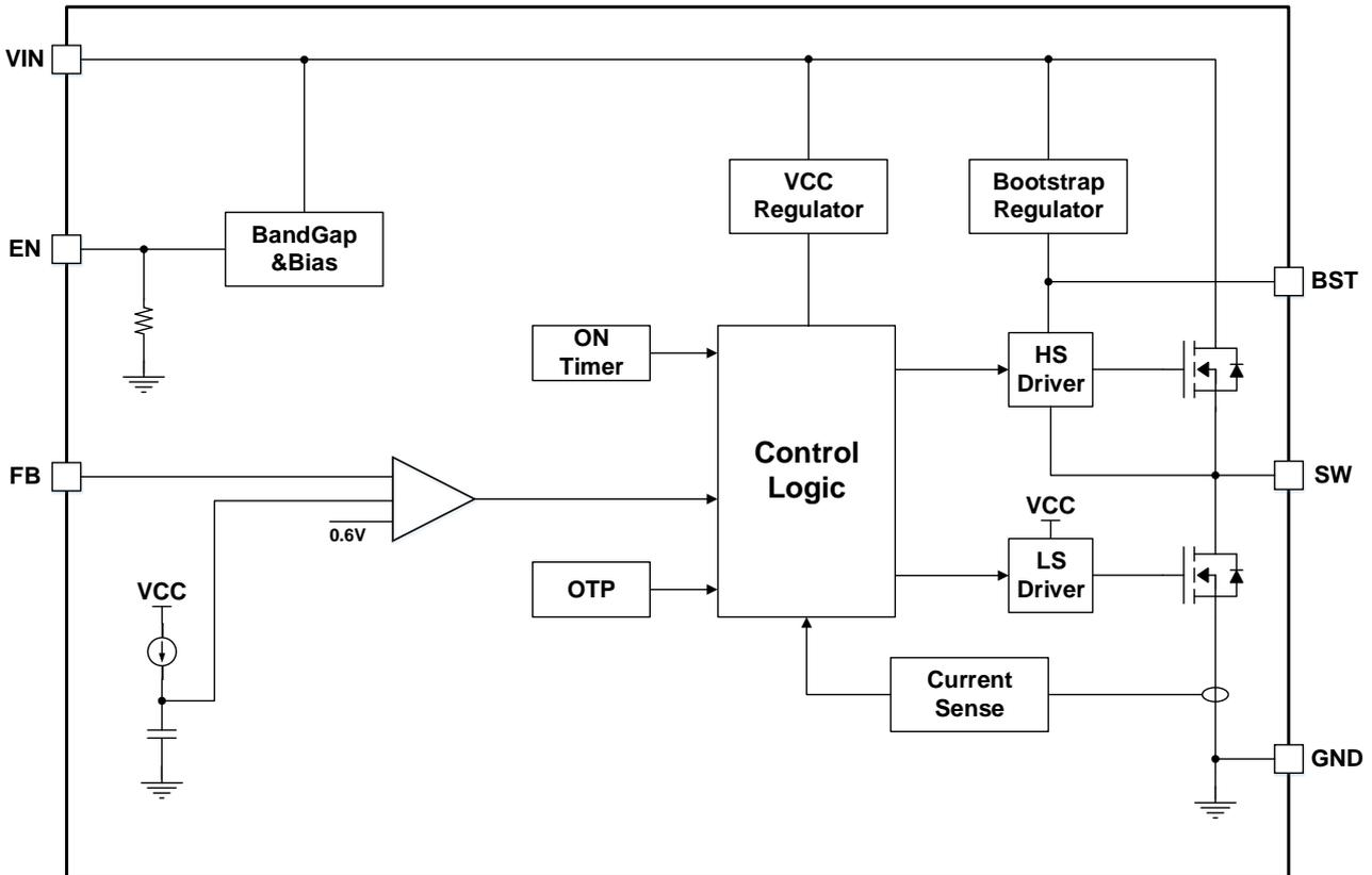
Figure 1. GD30DC1350 Functional Block Diagram
