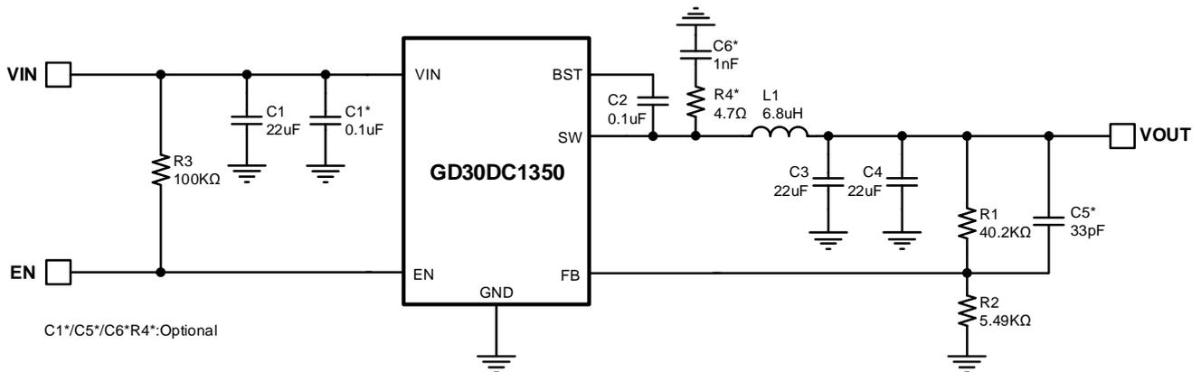
Figure 2. 5.0V, 3A Reference Design
