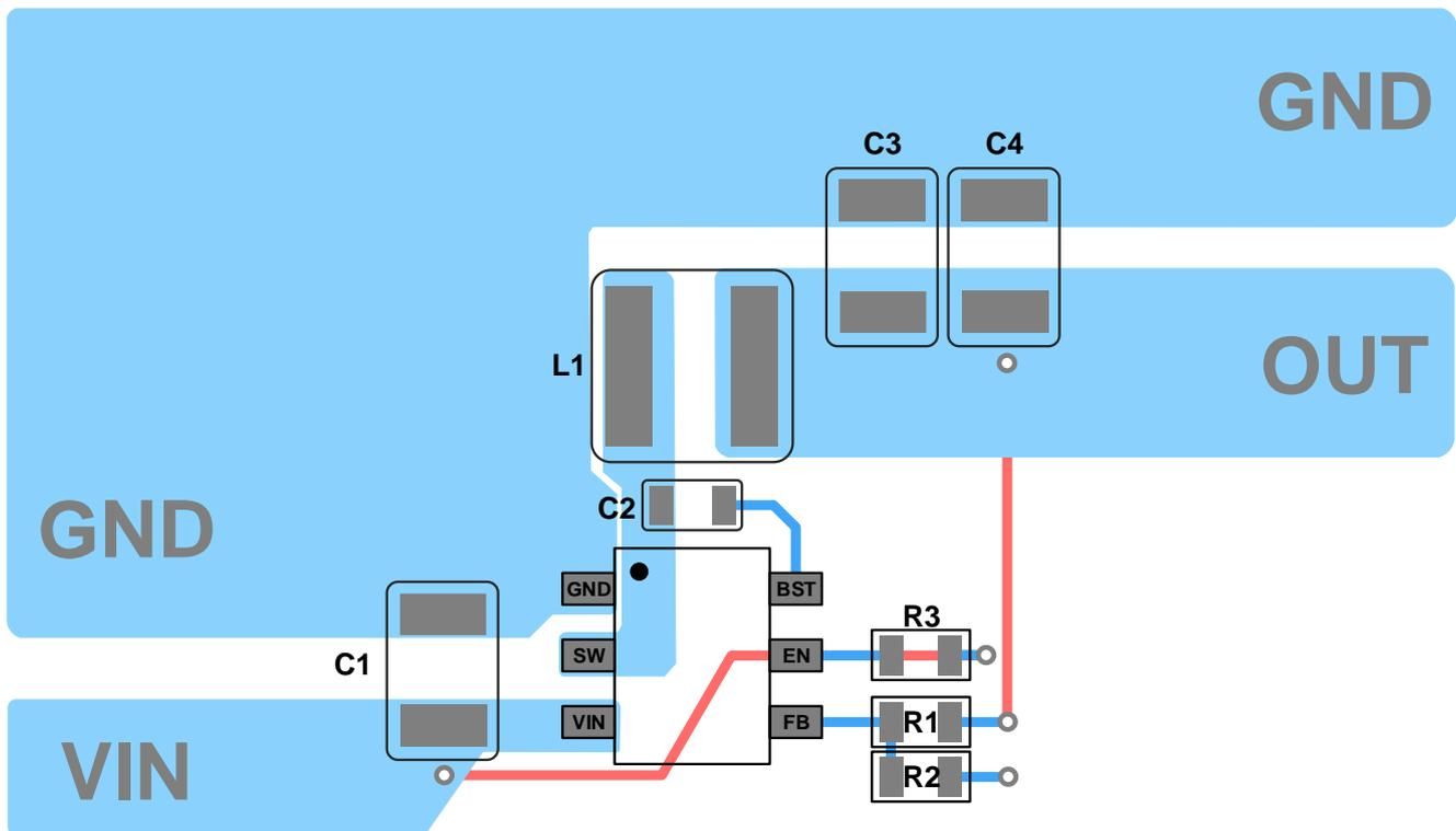
Figure 4. Typical GD30DC1350 Example Layout
