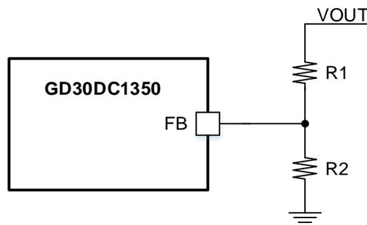
Figure 3. Feedback resistor divider
