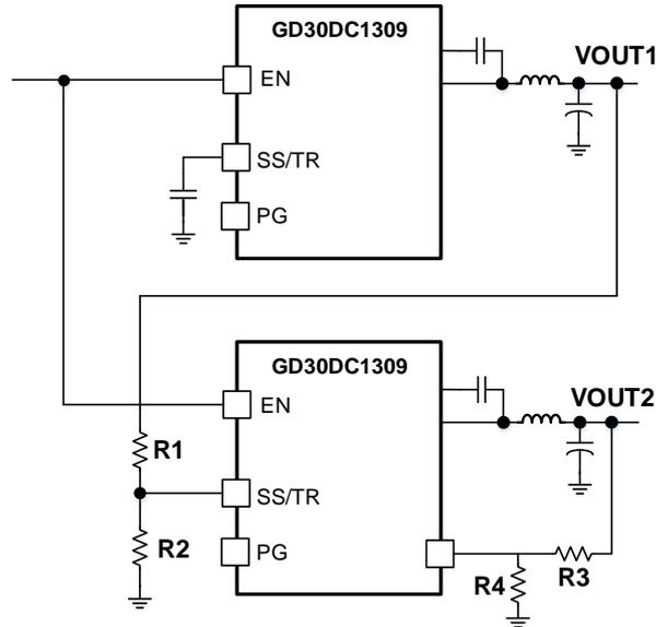
Figure 15. Ratiometric and Simultaneous Start-Up Sequence
