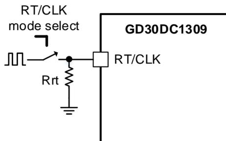
Figure 12. Using RT and CLK Modes Together
