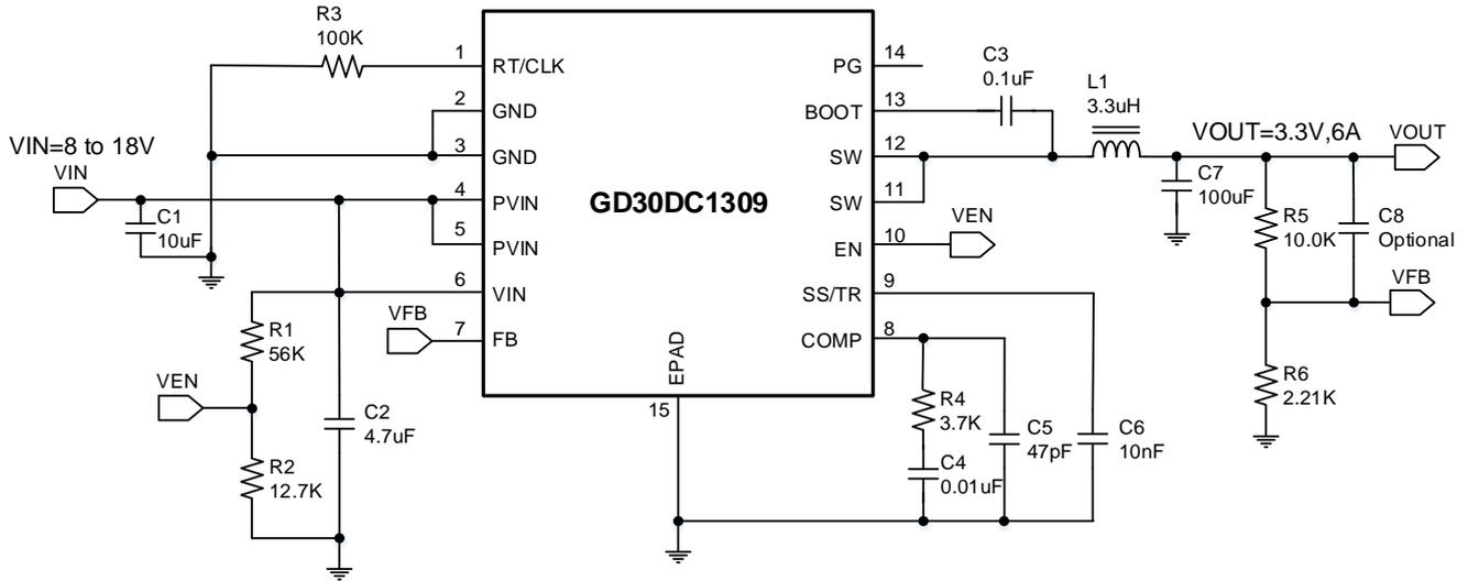
Figure 16. 3.3V, 6A Reference Design
