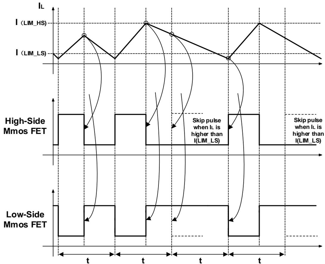
Figure 6. Overcurrent Protection for Both MOSFETs
