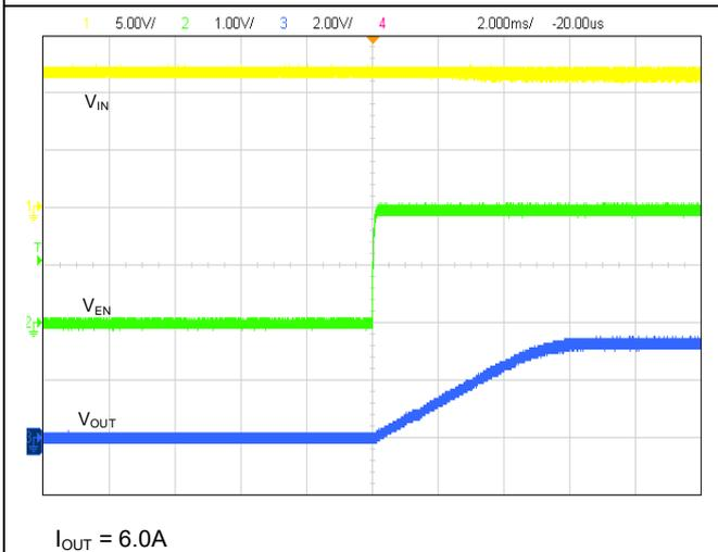
Figure 19. EN Startup with Load
