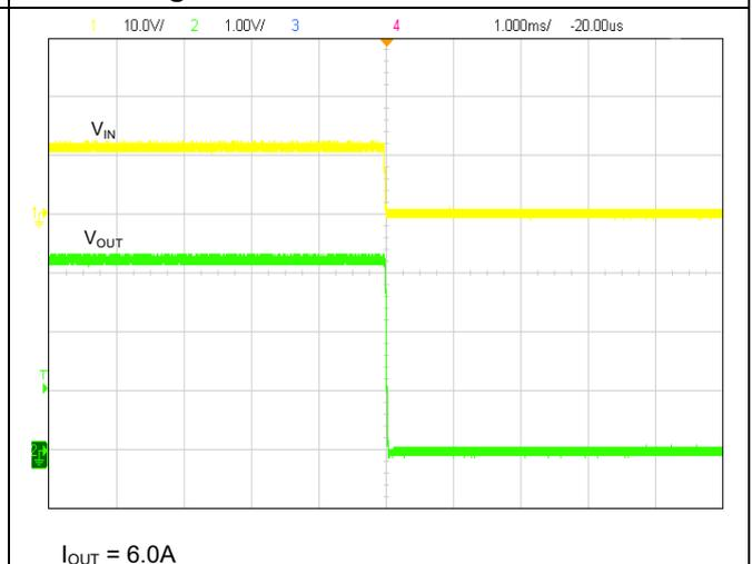
Figure 22. VIN Shutdown with Load
