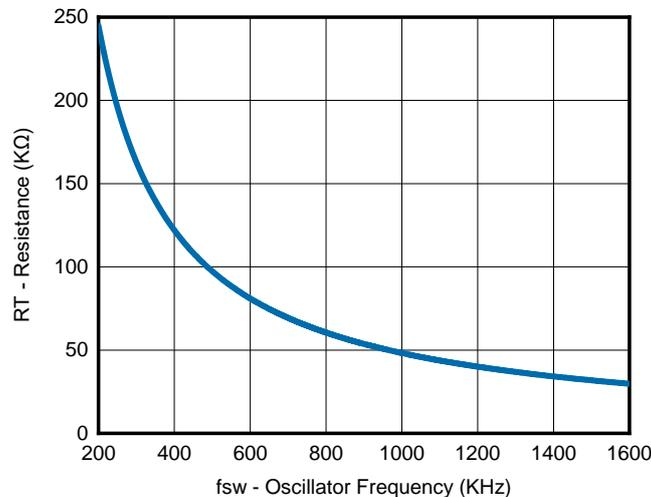
Figure 11. RT Set Resistor vs. Switching Frequency
