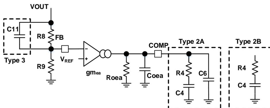
Figure 10. Types of Frequency Compensation
