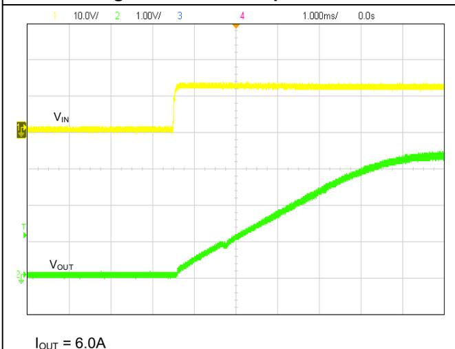
Figure 21. VIN Startup with Load
