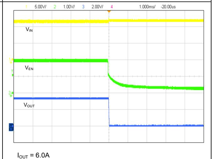
Figure 20. EN Shutdown with Load
