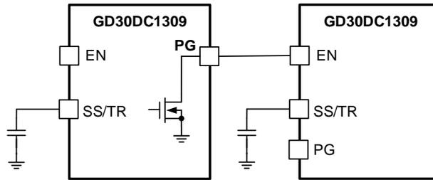
**Figure 13. Sequential Start-Up Sequence**
