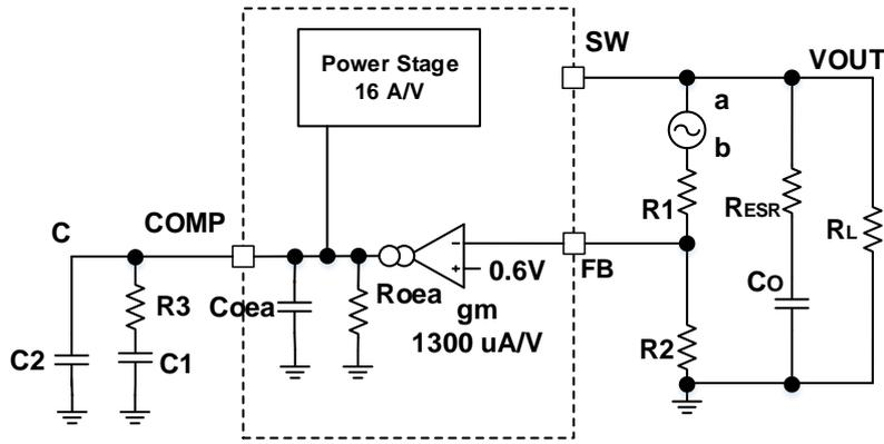
Figure 7. Small Signal Model for Loop Response
