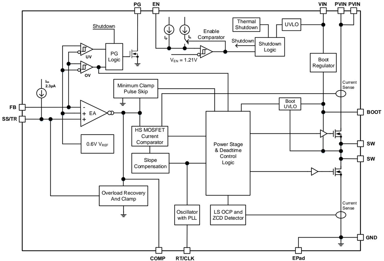
Figure 1. GD30DC1309 Functional Block Diagram
