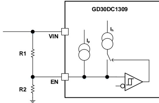
Figure 4. PVIN UVLO Setting ( $V_{IN} \geq 4.5V$ )
