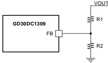
Figure 2. Feedback resistor divider diagram
