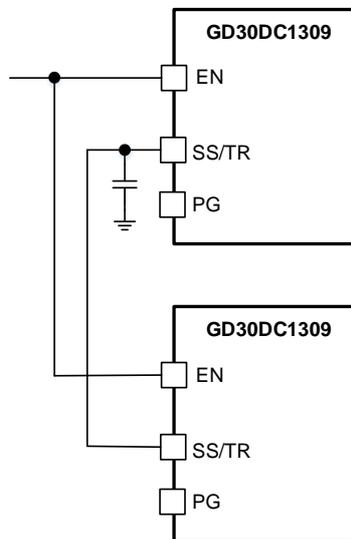
**Figure 14. Ratiometric Start-Up Sequence**
