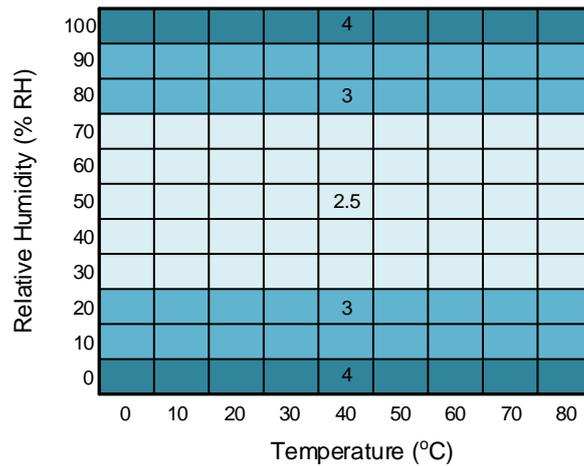
Figure 2. Typical RH Accuracy Tolerance Over Humidity and Temperature for GD30TSHTV4
