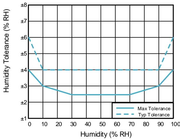
Figure 1. Tolerance of RH @25°C for GD30TSHTV4
