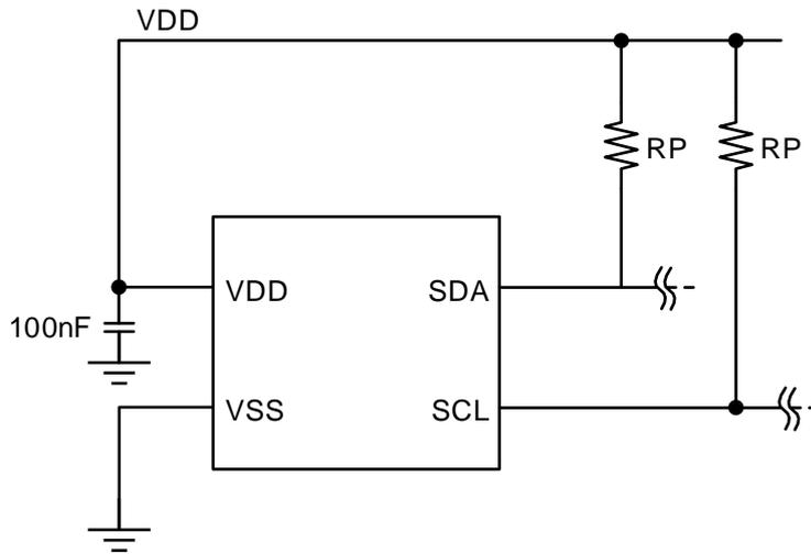
Figure 6. GD30TSHTV4 Reference Circuit
