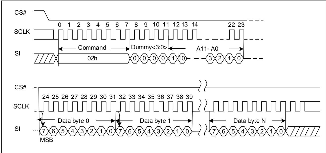
Note: When internal ECC disabled the Data Byte is 2176, when internal ECC enabled the Data Byte is 2112.
