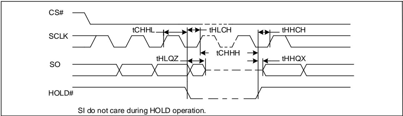
Figure 18-4. Serial Input Timing (DTR)
