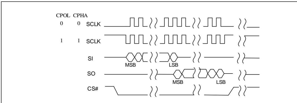
Note: While CS# is HIGH, keep SCLK at VCC or GND (determined by mode 0 or mode 3). Do not toggle SCLK until CS# is driven LOW.
