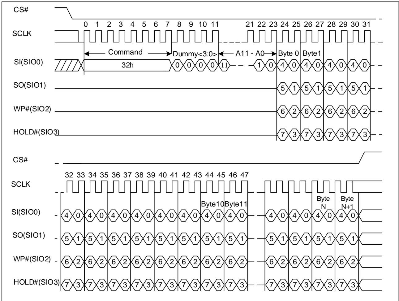
Note: When internal ECC disabled the Data Byte is 2176, when internal ECC enabled the Data Byte is 2112.
