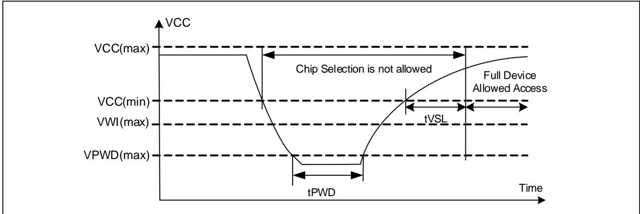
Table 13. Power-On/Off Timing and Write Inhibit Threshold for 1.8V/3.3V
